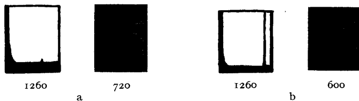
Fig. 1. Ultracentrifuge diagrams of T2 bacteriophage preparations. 1a. Untreated phage. 1b. Phage after colloid mill treatment. Sedimentation proceeds to the left. The right-hand diagram in each experiment was taken at a rotor speed of 9,000 r.p.m.; the left at 47,520 r.p.m. The time in seconds after the rotor had attained the appropriate speed is given under each diagram. The experiments were performed in buffer I.
